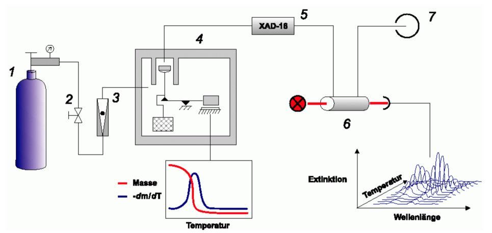
1 synthetic air bottle with pressure controller, 2 high precision flow regulator,
