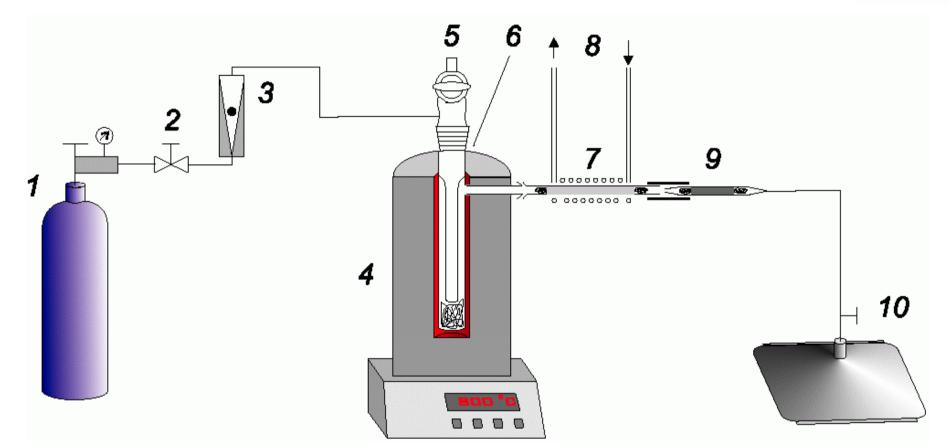
synthetic air bottle with pressure controller, 2 high precision flow regulator,
